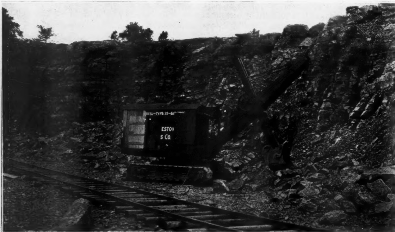
Electric Shovel Loading Dump Cars in Quarry
